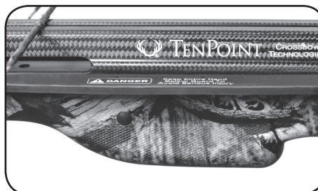
Safety wings are bedded between the stock and barrel. They help prevent thumb and finger injury and they dampen noise.
