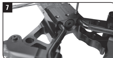
Once the foot stirrup is in place, tighten all three setscrews. See below if mounting the 3-Arrow Instant Detach Quiver.
